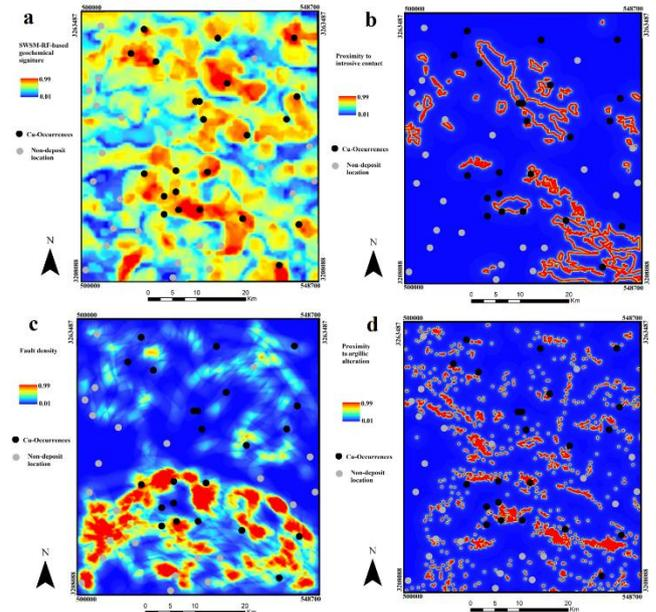
Fig.3. Derived evidence layer from exploration data (a) SWSM-based multi-element geochemical signature (b) proximity to intrusive contacts (c) fault density (d) proximity to argillic alteration.
