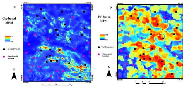
**Fig.4.** Prospectivity map for porphyry-Cu deposits generated through integrating multiple evidence layers using (a) Geometric average function (b) random forest algorithm.
