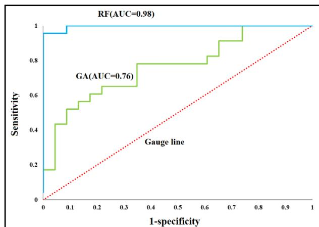
**Fig.5.** ROC plots for the evaluation capabilities of random forest algorithm and geometric average function for mineral prospectivity modeling.
