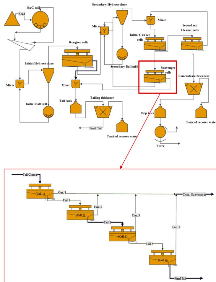
Fig. 1. Schematic illustration of scavenger flotation circuit of phase 1 of the Sungun copper concentration plant.
