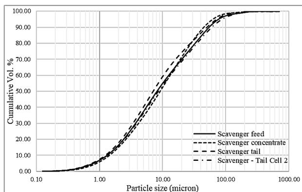
Fig. 2. Particle size distribution diagrams of feed, concentrate, and tailings of the scavenger circuit of the Sungun copper concentrating plant.
