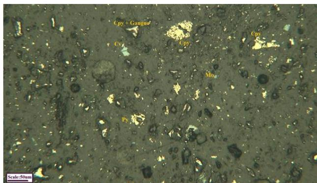
**Fig. 4.** Copper minerals and their distribution in the flotation test concentrate - Sungun copper scavenger circuit (Cpy: chalcopyrite, Mo: molybdenite, Py: pyrite).
