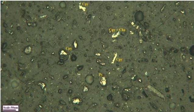
**Fig. 3.** Abundance and distribution of copper minerals in flotation test concentrate obtained from the scavenger circuit of the Sungun copper concentration plant (Cpy: chalcopyrite, Cha: chalcocite, Py: pyrite).
