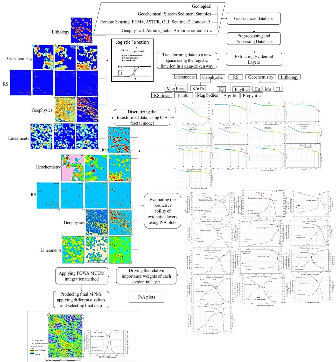
Fig. 2. A schematic flowchart of porphyry Cu potential mapping through a hybrid FOWA method.
