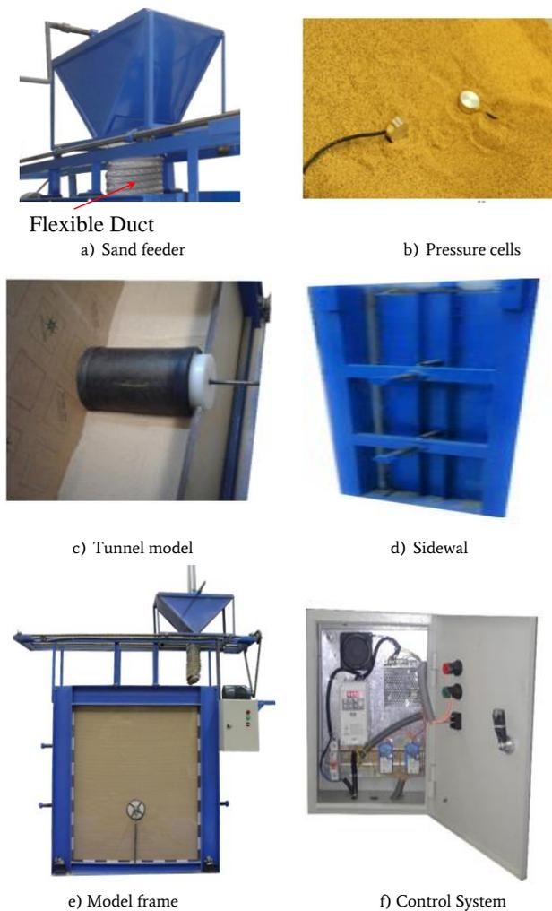
Figure 1. Physical model of the full-face tunnel excavation.
