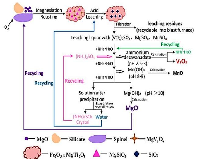
Figure 17. The flowsheet of magnesian roasting-acid leaching with multiple recycling [16]
