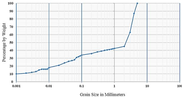
Fig. 6. Soil particle distribution of investigated wall.
