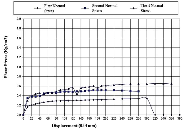
Fig. 7. Shear stress against displacement in small scale.
