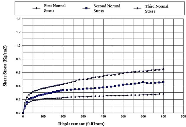
Fig. 8. Shear stress against displacement in large scale.
