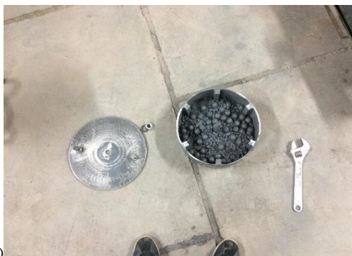
Figure 2. a) The Starkey mill made in our lab, b) The Starkey mill on the rolls.
