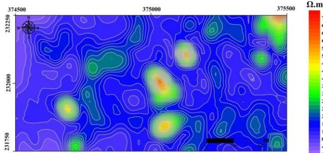
Figure 5. Result of geo-electrical mapping. The disturbed areas are surrounded by red circles.
