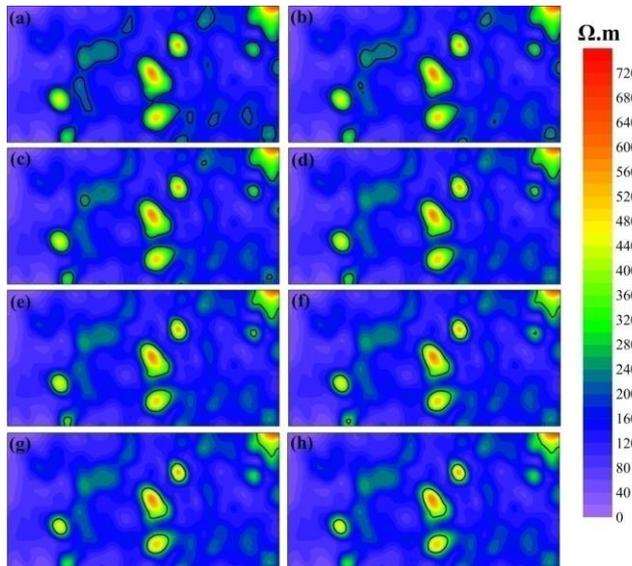
Figure 6. Geo-electrical images showing the spatial distribution of the disturbances over the study area. The cutoff frequencies  $v_{ar}$  used of each image are: (a)  $v_{ar}=200\Omega.m$ , (b)  $v_{ar}=220\Omega.m$ , (c)  $v_{ar}=240\Omega.m$ , (d)  $v_{ar}=260\Omega.m$ , (e)  $v_{ar}=280\Omega.m$ , (f)  $v_{ar}=300\Omega.m$ , (g)  $v_{ar}=320\Omega.m$ , (h)  $v_{ar}=340\Omega.m$ .
