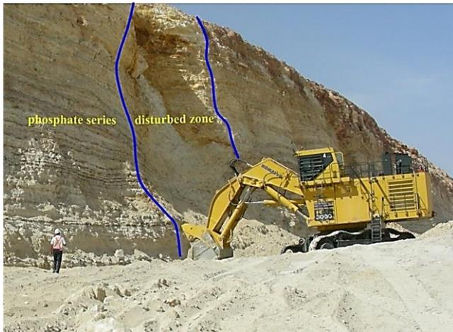
Figure 2. Geological sections showing disturbed zone in Sidi Chennane mine.
