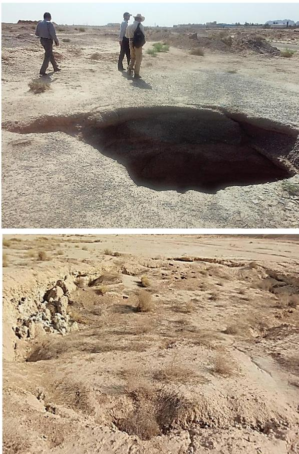
**Fig. 5.** Creating deep cracks, cavities, and circular structures on the ground around Abarkuh as pieces of evidence of sinkhole occurrence.
