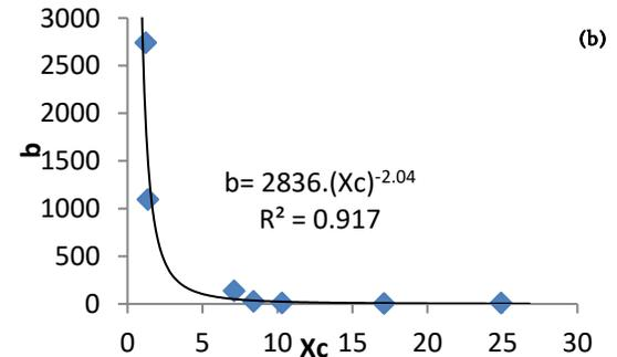
Fig. 12. undulating parameters  $b$  of Swebrec against Rosin-Rammler parameters (a)  $n$  and (b)  $X_c$
