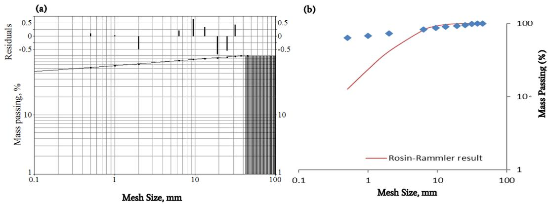
Fig. 8. Mass passing % vs sieve sizes for Sandstone from blast test, (a) Swebrec and (b) Rosin-Rammler
