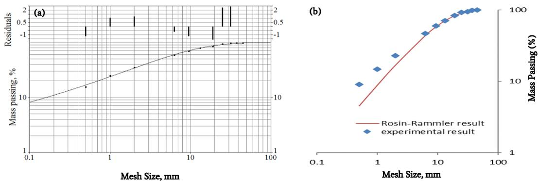
Fig. 5. Mass passing % vs sieve sizes for coarse-grain Granite from blast test, (a) Swebrec and (b) Rosin-Rammler
