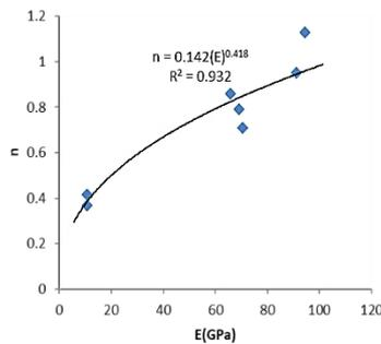
Fig. 15. uniformity index of Rosin-Rammler, n against Elastic parameter E (GPa)
