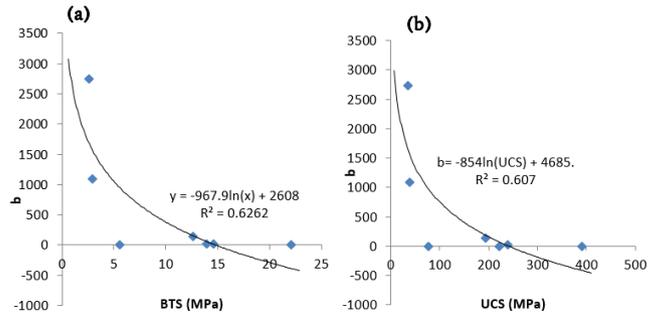
Fig. 18. undulation parameters b of Swebrec against Strength properties (a) BTS and (b) UCS
