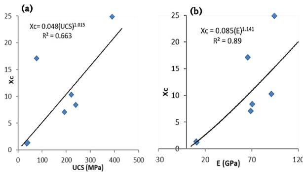
Fig. 14. characteristic size, Xc of Rosin-Rammler against (a) UCS and (b) E
