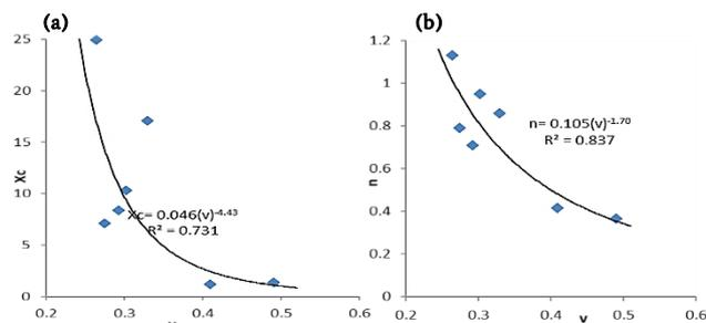
Fig. 16. Poisson's ratio  $\nu$  against (a) characteristic size and (b) uniformity index of Rosin-Rammler
