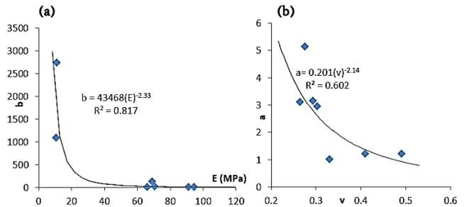
Fig. 19. undulation parameters b and factor a of Swebrec against elastic parameters (a) E and (b)  $\nu$
