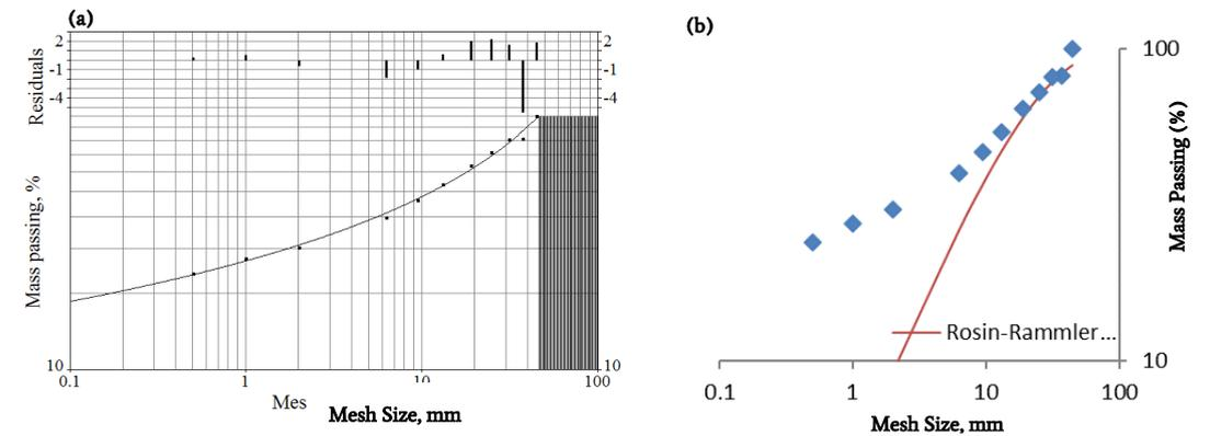
Fig. 7. Mass passing % vs sieve sizes for Marble from blast test, (a) Swebrec and (b) Rosin-Rammler
