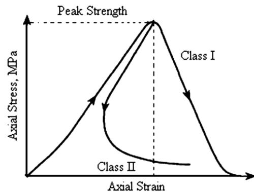
**Fig.1.** Classification of rock into Class I and Class II behavior in uniaxial compression tests [14]
