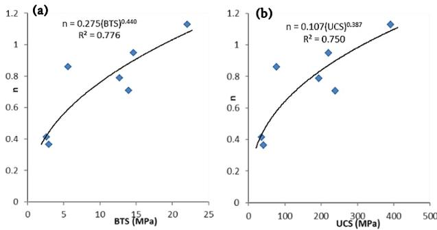
Fig. 13. uniformity index of Rosin-Rammler, n against Strength properties (a) BTS and (b) UCS
