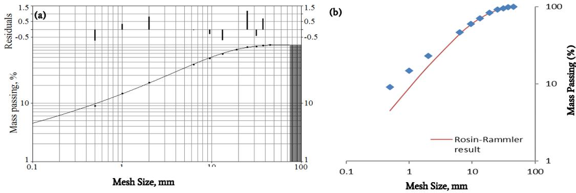
Fig. 4. Mass passing % vs sieve sizes for Norite from blast test, (a) Swebrec and (b) Rosin-Rammler
