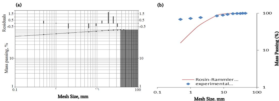
Fig. 9. Mass passing % vs sieve sizes for Feldspathic arenite from blast test, (a) Swebrec and (b) Rosin-Rammler
