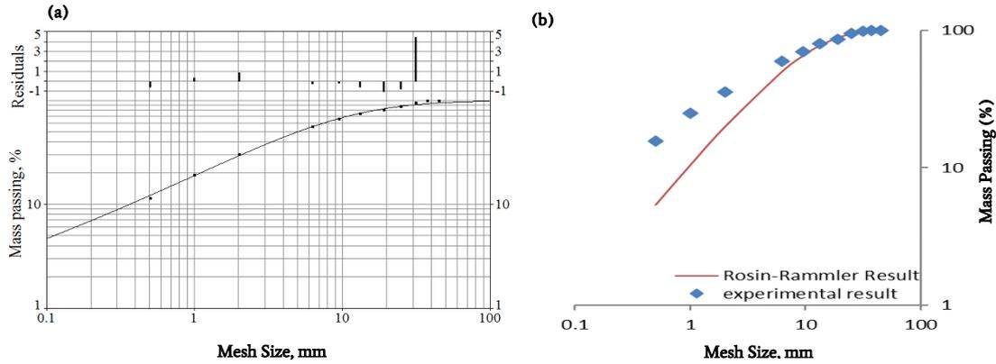
Fig. 6. Mass passing % vs sieve sizes for fine-grain Granite from blast test, (left) Swebrec and (right) Rosin-Rammler
