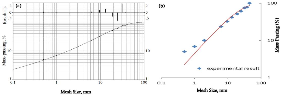
Fig. 3. Mass passing % vs sieve sizes for Gabbro from blast test, (a) Swebrec and (b) Rosin-Rammler
