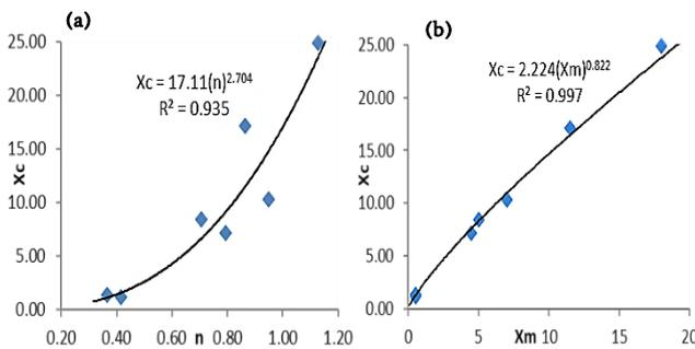
Fig. 10. Characteristic size,  $X_c$  against (a)  $n$  and (b)  $X_m$
