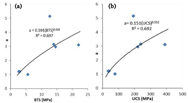
Fig. 17. factor 'a' parameters of Swebrec against Strength properties (a) BTS and (b) UCS
