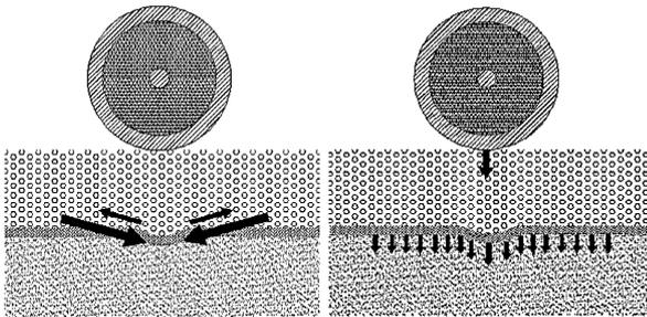
Fig. 1: Function of Geogrids in Flexible Road Pavement [7]
