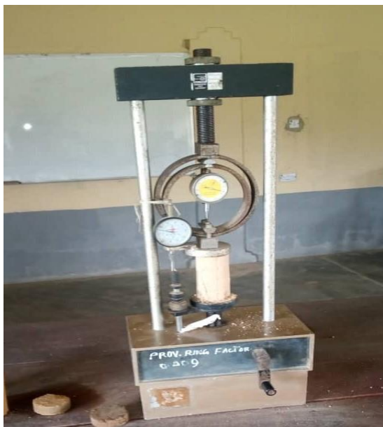
Fig. 3: Unconfined compressive strength experimental setup
