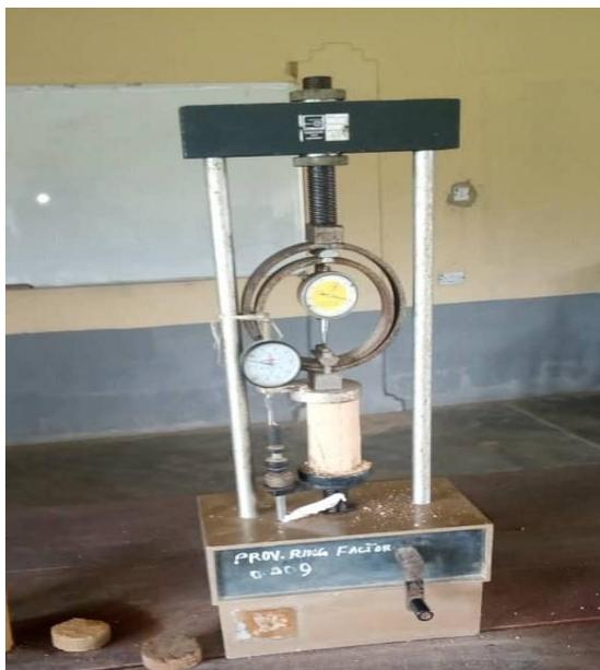
Fig. 3: Unconfined compressive strength experimental setup
