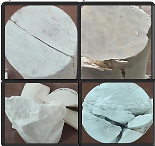
Fig5. Thermal breakage of Ghulmet marble specimens
