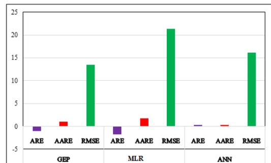
Figure 7. Comparison of the statistical parameters for predictions of MLR, ANNs, and GEP models
