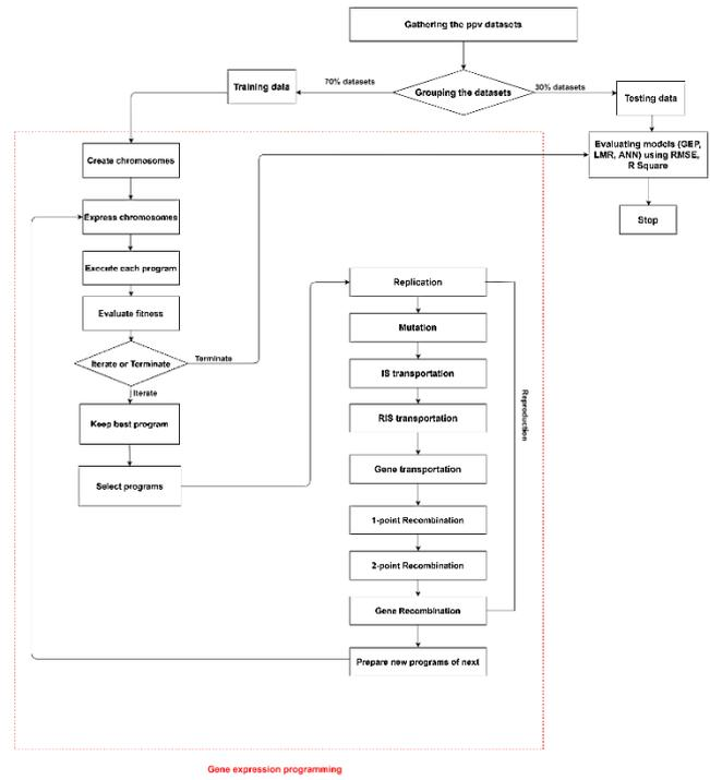
Figure 1. Flowchart of GEP algorithm
