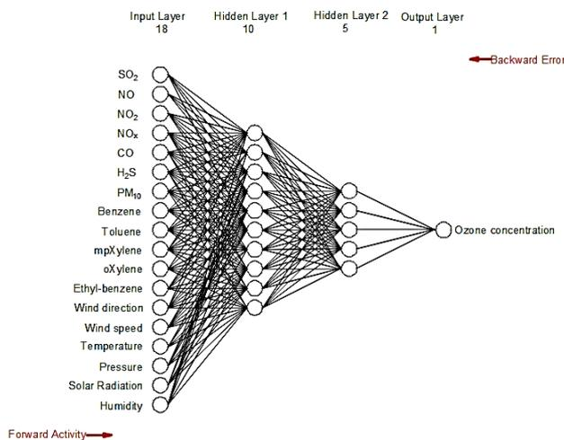
Figure 5. the ANNs architecture with 18-10-5-1 (back-propagation network)
