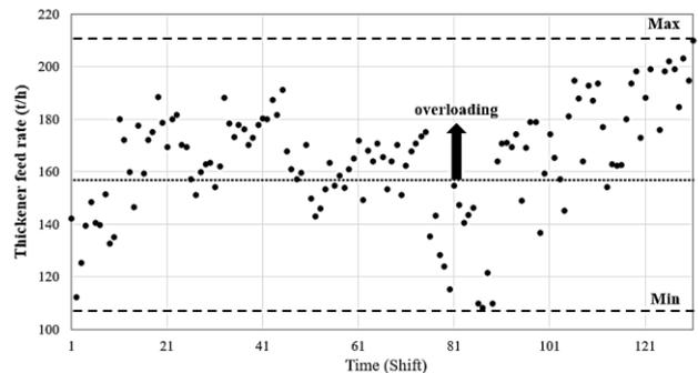
**Figure 2.** Thickener feed rate (t/h) in 130 shifts
