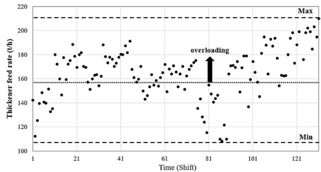
**Figure 2.** Thickener feed rate (t/h) in 130 shifts
