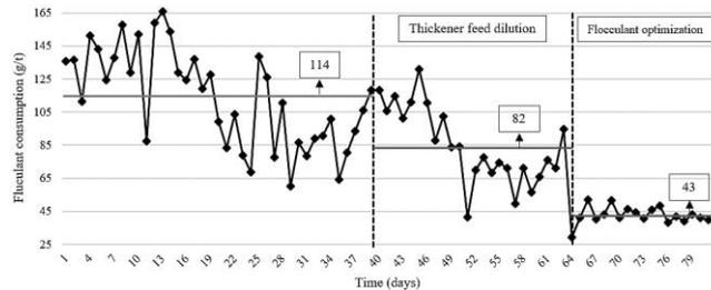
Figure 12- Flocculant consumption before and during modifications
