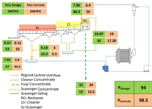
Fig. 5- Mass balanced data for the cleaner, reclaimer, and scavenger stages.
