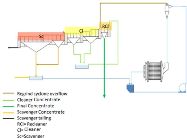
Fig. 6- Part of the layout of the flotation circuit (initial plant design)
