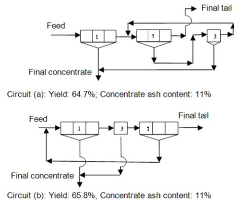
Fig. 1- Effect of flotation circuit configuration on efficiency [3]
