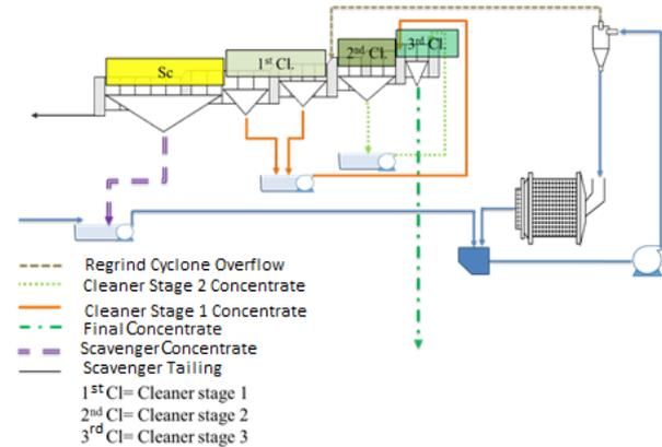
Fig. 7- Part of the layout of the flotation (after adding a cleaner stage).
