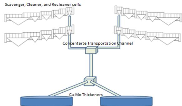
Fig. 3- Schematic design of the gravity transportation of the final concentrate.
