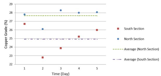
Fig. 8- Final copper concentrate grade in the north (new layout) and south sections (old layout).
