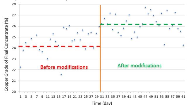
Fig. 9- Final copper concentrate before and after modifications.
