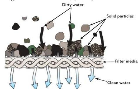
Figure 1. Mechanism of cake formation in the filtration process.
