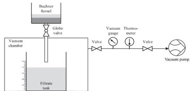
Figure 4. Operational apparatus of filtration process in Lab.
