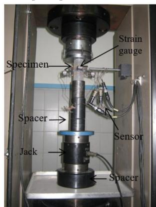
Fig 6. The uniaxial compressive strength apparatus
