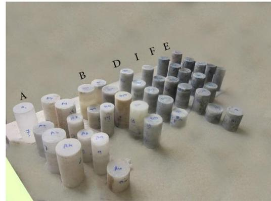
**Fig 3.** Categorizing salt rock samples based on the impurity content.
