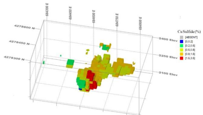
**Fig. 12.** The 3D model of Cu grade made from the integration of IP and Rs anomalous zones.
