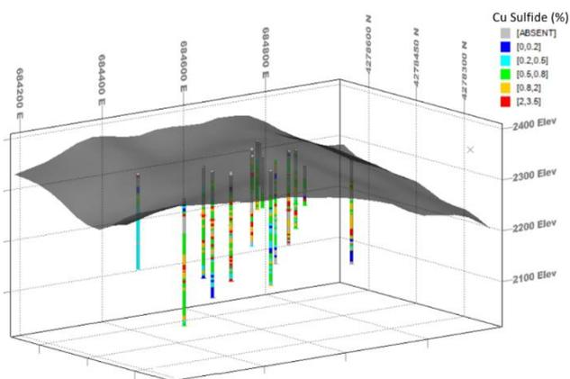
Fig. 4. Location of boreholes with respect to the topographic surface in the study area. Cu grades are shown along each borehole as well.
