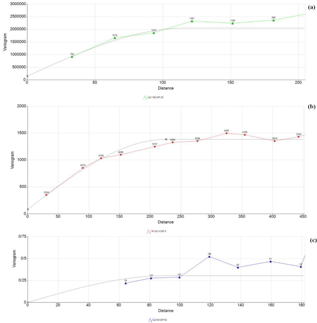
Fig. 9. Experimental directional semi-variogram models, and the number of pairs for (a) the electrical resistivity, (b) induced polarization, and (c) Cu grade.
