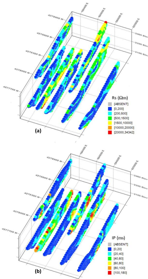
Fig. 5. 3D visualization of all 2D inverted profiles of electrical resistivity (a), and chargeability (b).
