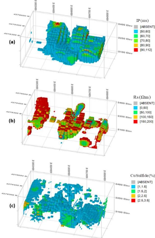
**Fig. 11.** 3D models of induced polarization (a), resistivity (b), and Cu Sulfide content (c) in the study area. Threshold values were assumed equal to 50-112 ms, less than 200 Ohm.m, and higher than 1.1 %, respectively.
