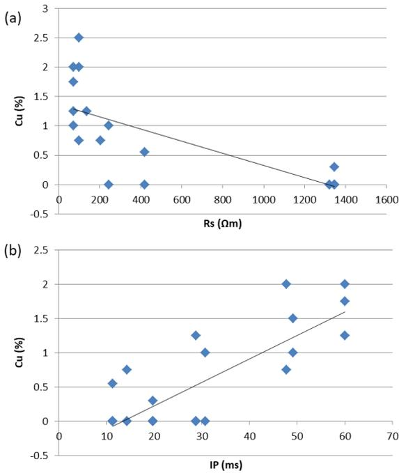
Fig. 7. Scatter plots of Cu grades along the borehole near the ERT survey versus the electrical resistivity (a) and chargeability (b) for profile 4.
