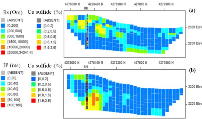
Fig. 6. A cross-section view of the 2D inverted models of the electrical resistivity (a), and the induced polarization (b) along profile 4, on which Cu grades along the drilled borehole next to the ERT survey are overlain on the sections.
