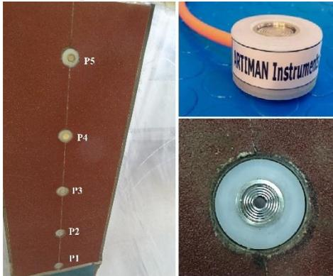
Fig. 4. Miniature pressure cells installed in thick rigid wall.
