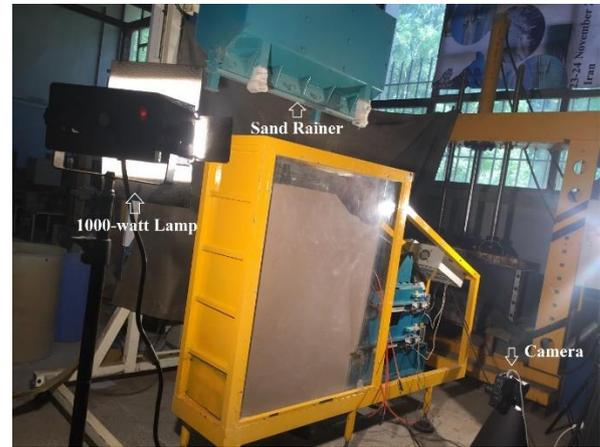
Fig. 5. Physical model box, sand rainer, and shooting equipment.
