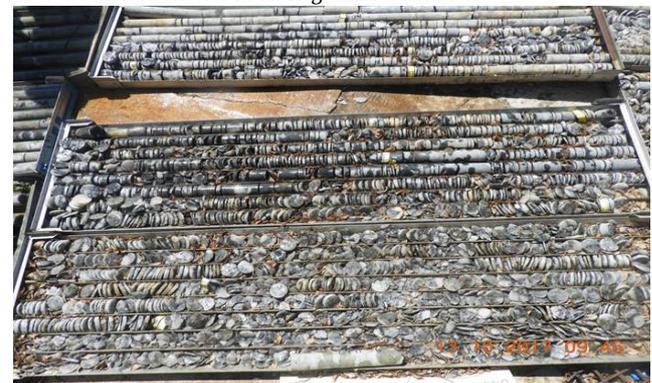
**Fig. 11.** Extensively crushed core recovered ahead of the mining flank.
