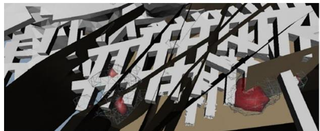
Fig. 17. Higher risk of strain bursting in the walls, rather than at the face.
