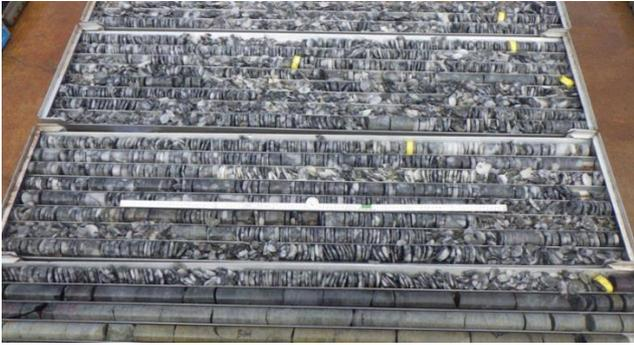
Fig. 12. Crushed core recovered ahead of the leading drive.
