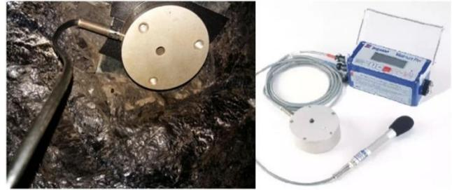
**Fig. 2.** Monitoring tool of the blasting vibrations and a geophone installed on the stope's roof.
