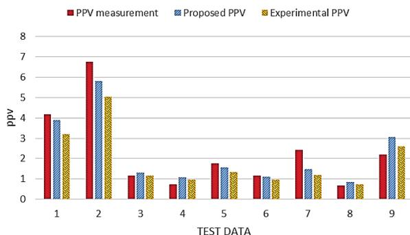
Fig. 7. comparative diagram of PPV calculated by the empirical equation, proposed equation, in-situ measurement values.
