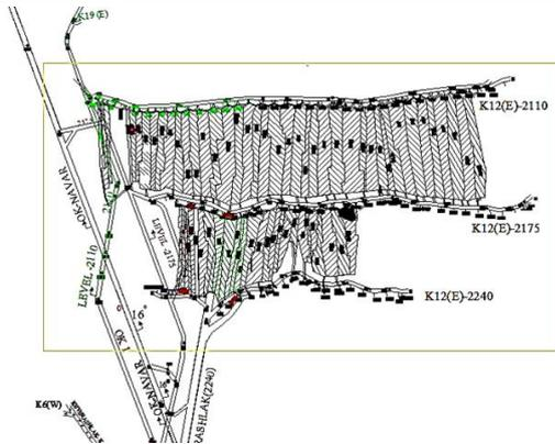
**Fig. 1.** The position of the development tunnels and the stope face in the seam K12 of the Alborz-e-Sharghi coal mine.
