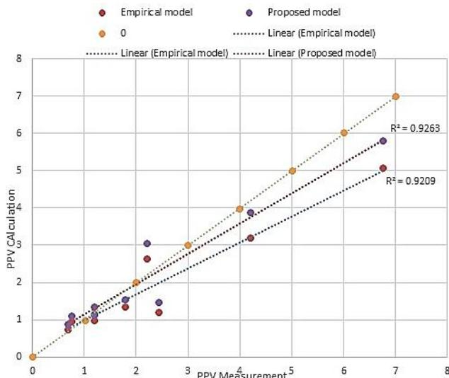
Fig. 6. Comparison of the peak particle velocity measured and calculated from the experimental and suggested models.
