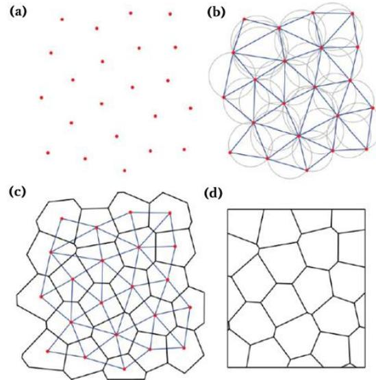
**Fig. 2.** Voronoi tessellation generator logic used in UDEC: (a) Random generation of points, (b) Creation of the Delaunay triangulation, (c) Generation of the Voronoi blocks and (d) Truncation of polygons at the boundary of the tessellation region [24].
