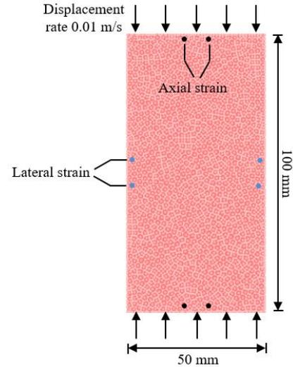
Fig. 5. Simulation of the uniaxial compression test.
