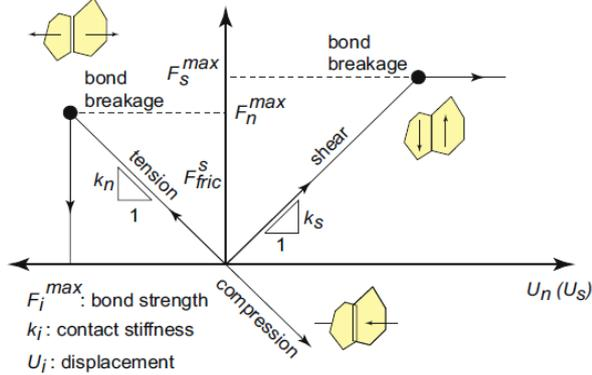
Fig. 4. The Coulomb contact slip model [27, 28].
