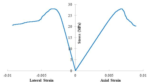
Fig. 6. Stress-strain curve of the calibrated numerical model.
