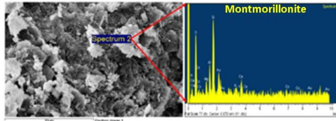
Fig. 8. SEM Photomicrograph and EDX semi-qualitative analysis on sample K3.
