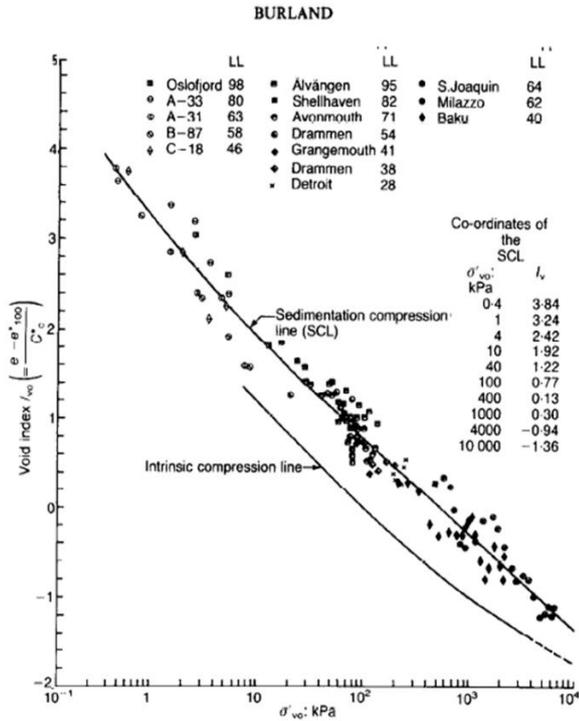
Fig. 5. Relationship between  $I_{v0}$  and  $\log \sigma'_{v0}$  for many of the normally consolidated clays.
