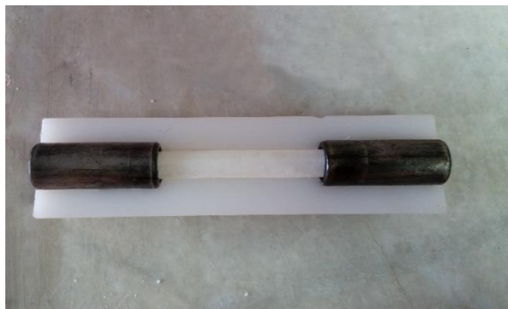
Fig. 5. Prepared specimen consisting the rock sample and steel frames.
