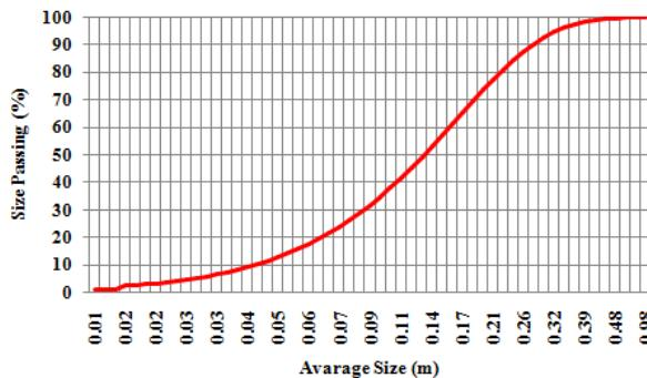
**Fig. 2.** Distribution curve for a blast, the Chadormalu iron ore mine.
