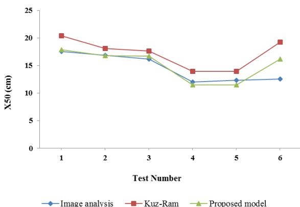
**Fig. 4.** Comparison of the mean fragment size of image processing, the proposed and the Kuz-Ram models in the Chadormalu iron ore mines.
