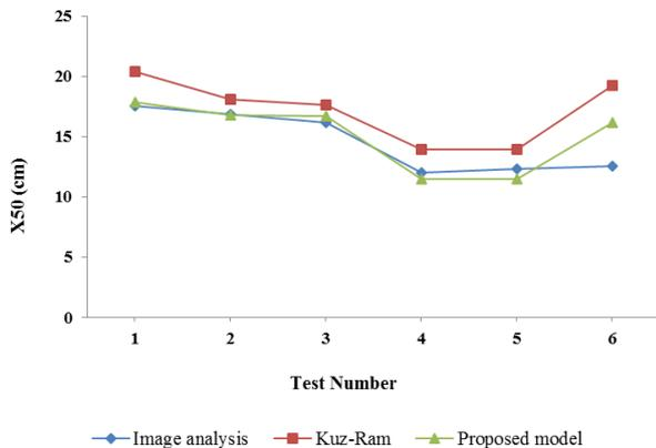
Fig. 4. Comparison of the mean fragment size of image processing, the proposed and the Kuz-Ram models in the Chadormalu iron ore mines.
