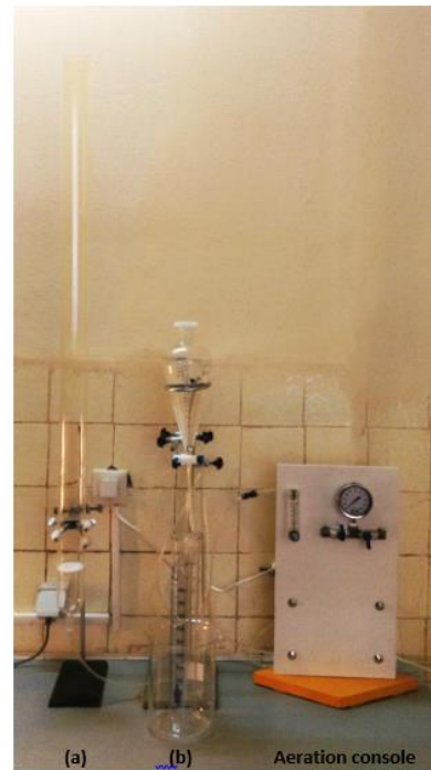
Figure 8. Comparison between dimensions of column frothmeter (a) and set-up used for water recovery measurement in this research study (b).
