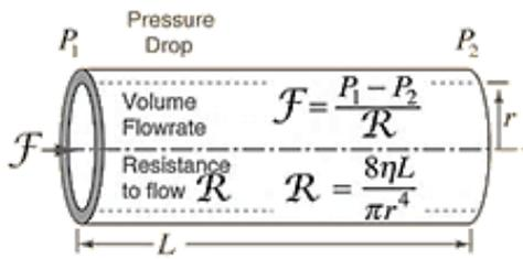
Figure 1. Considered cylinder for fractures flow modeling
