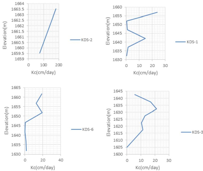
Diagram 1. Hydraulic conductivity values of Lufran analysis in alluvium aquifers.
