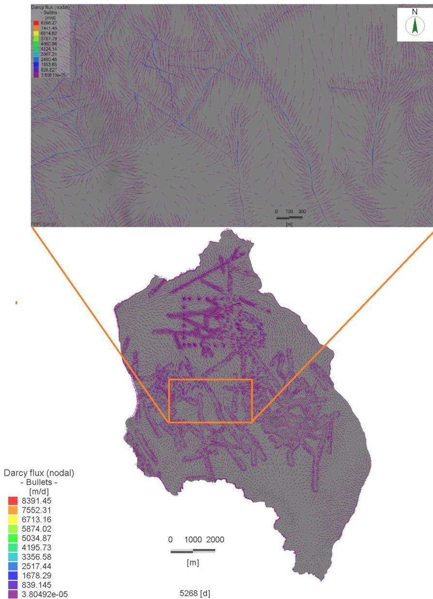
Figure 12. The direction of flow calculated through numerical modelling (Darcy flow velocity model).
