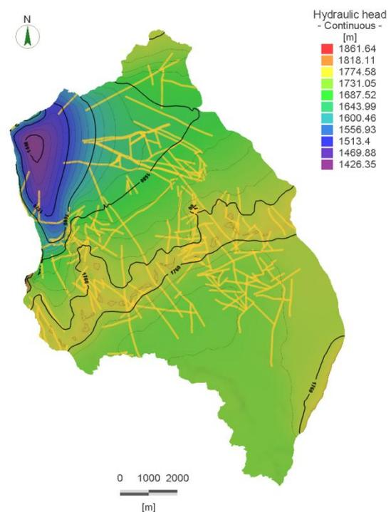
Figure 8. The values of water table level calculated from the transient model in 2014.
