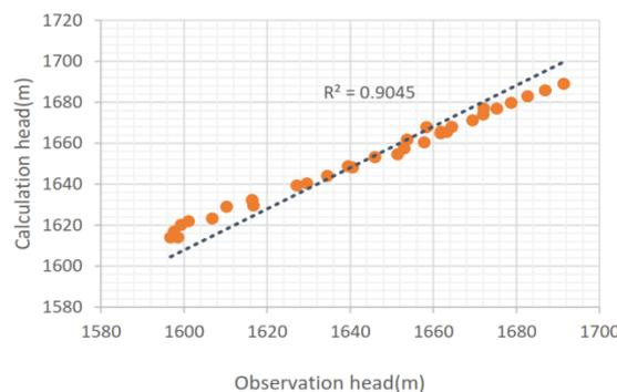
Diagram 3. Observed and calculated water table level in fall 2014 (5088 days).
