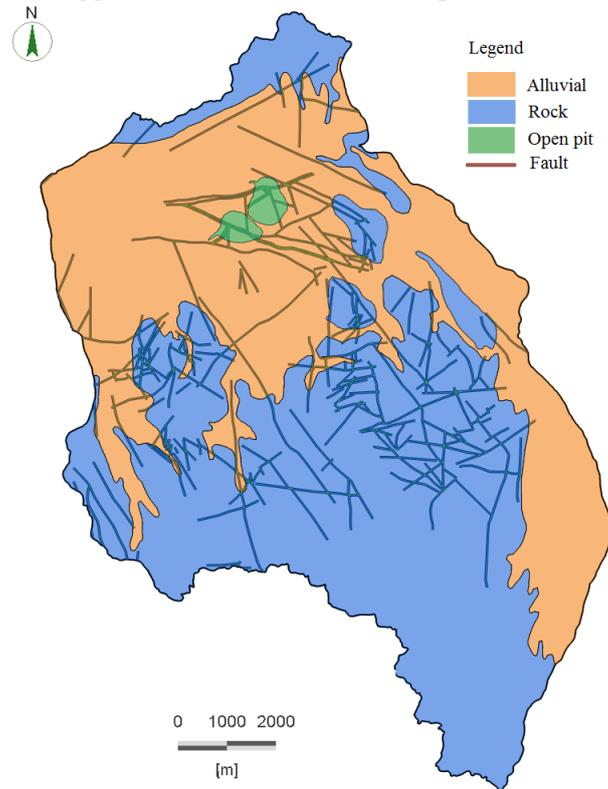
**Figure 6.** Separation of lithic and alluvium parts for determining the permeability, and hydraulic conductivity, the pit's location.
