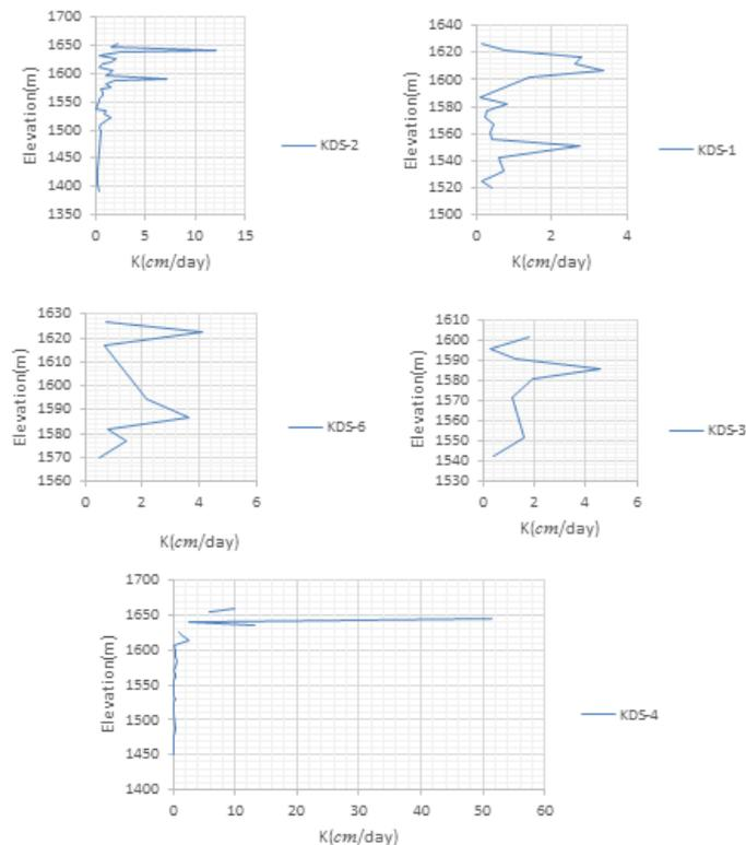
Diagram 2. Hydraulic conductivity values of Logan analysis in lithic systems.
