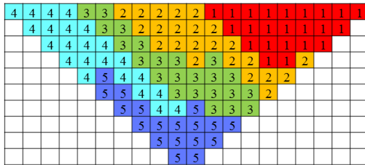
Figure 13. Mine production planning by mathematical method (The numbers are indicative of block extraction year).
