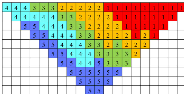
Figure 14. Mine production planning by ICA method (The numbers are indicative of block extraction year).
