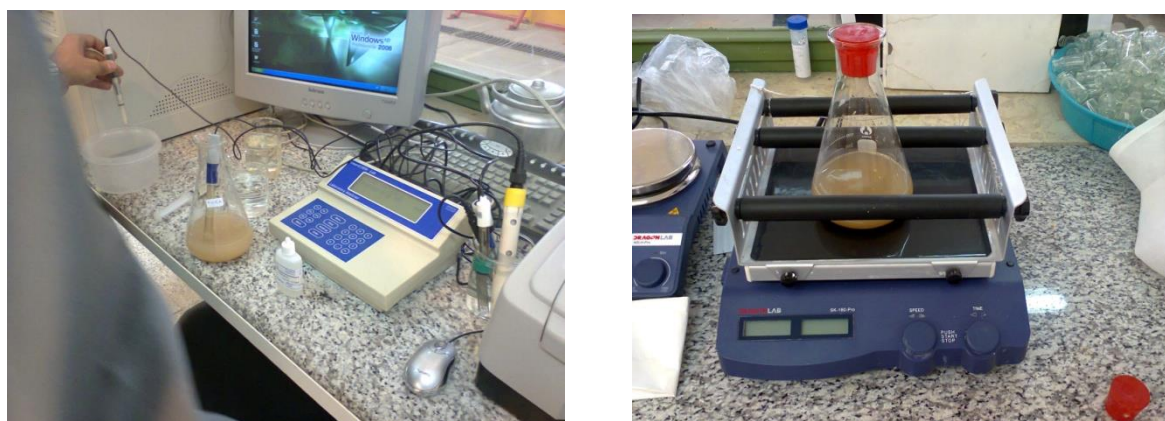
Fig. 2. The digital shaker (right) and the ion-meter (left) used in the study for measurement of pH and the concentration of chlorine
