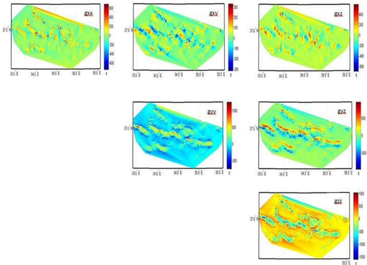
Fig. 3. Variations of the independent elements of the gravity gradient tensor in the study area by Fourier transform
