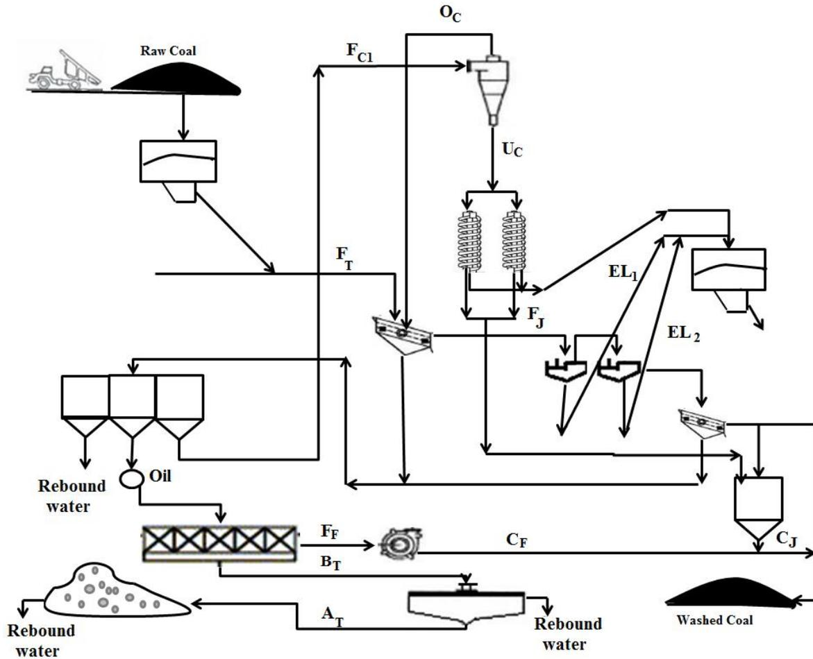
Fig. 1. Processing circuit of the Alborz-Sharghi coal washing plant
