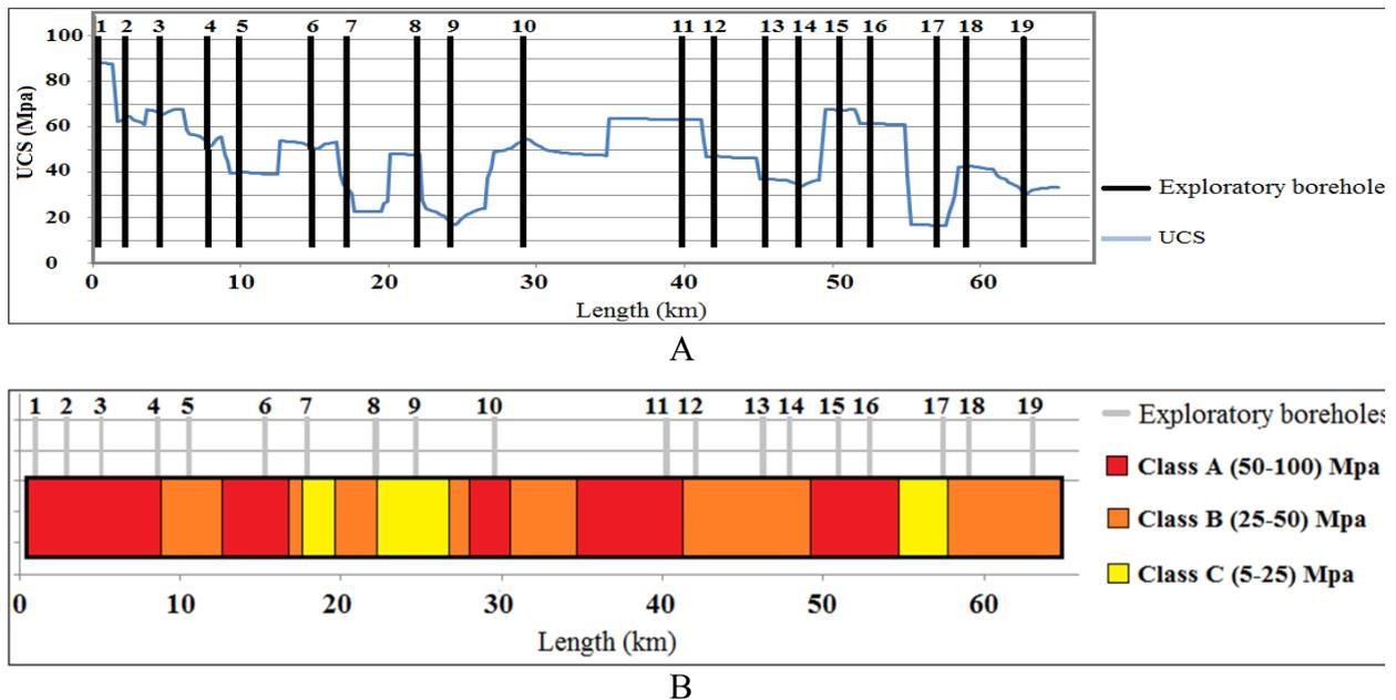
Fig. 10. a) geostatistical estimation values of UCS along the tunnel axis, b) classification of geostatistical estimation results for UCS along the tunnel axis
