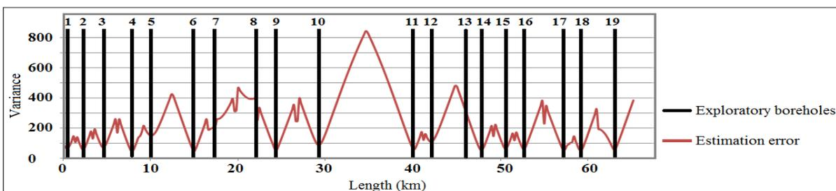
Fig. 9. Variance of estimation error along the tunnel axis
