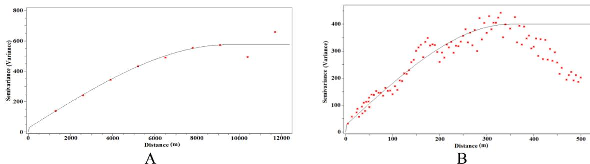
Fig. 4. A) Horizontal variogram of UCS values in the direction of the tunnel axis. B) Vertical variogram of UCS values.
