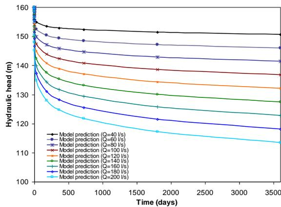
(e) Hydraulic head vs time for different Pumping out rates
