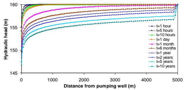
(b) Hydraulic head vs distance for pumping out test for various elapsed times on Bottom confined aquifer
