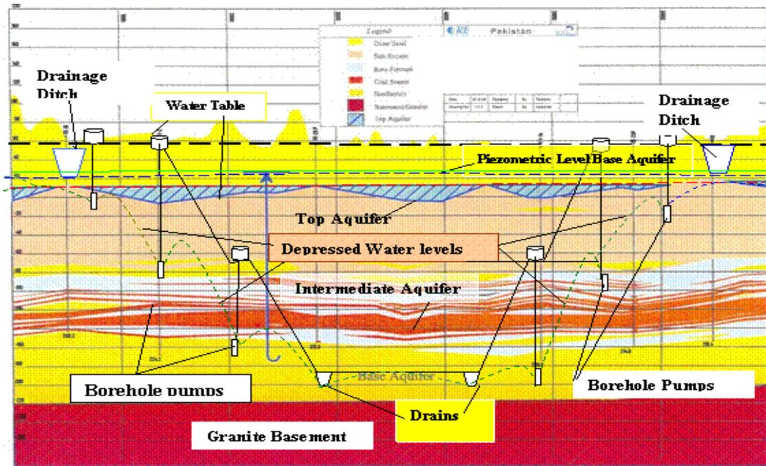
Figure 7. Dewatering arrangement of three aquifers in Thar lignite deposit [17].
