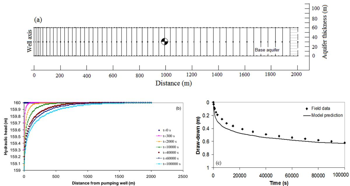
Figure 5. FE model of a pumping out well RE-52 with observation well RE-22 and the results of simulation. (a) Finite element model of well RE-52 Intersecting the Bottom aquifer, (b) Hydraulic head
