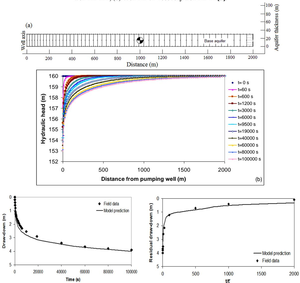
Figure 4. Comparison of field data with the computer model of pumping out test on well RE-51. (a) Finite element model of pumping well RE-51 in the Bottom aquifer, (b) Hydraulic head vs time for pumping out well RE-51 and Piezometric well RE-12P, (c) Comparison of model results with field data in RE-51
