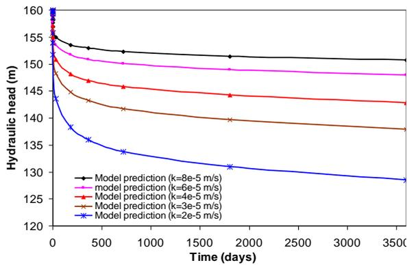
(c) Hydraulic head vs time for different permeabilities
