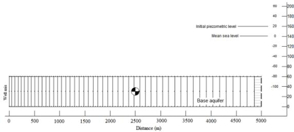
(a) Finite Element model of Thar Bottom aquifer
