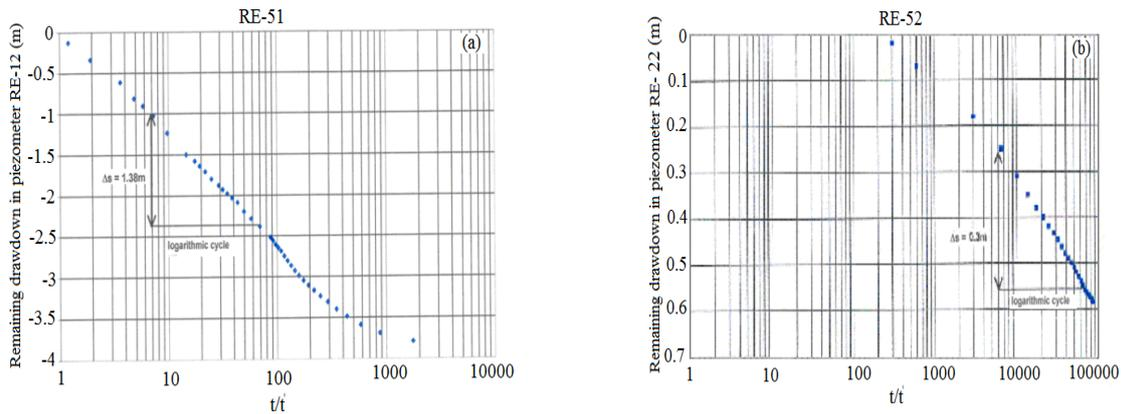
Figure 3. Results of pumping out tests in Thar lignite Prospect. (a) Pumping out Well RE-51W-recovery well RE-12P, (b) Well RE-52-recovery well RE-22 [3].
