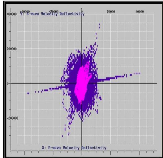
Figure 8: Crossplot between P-wave and S-wave Velocity Reflectivity in sub zone1 (Wet Zone)
