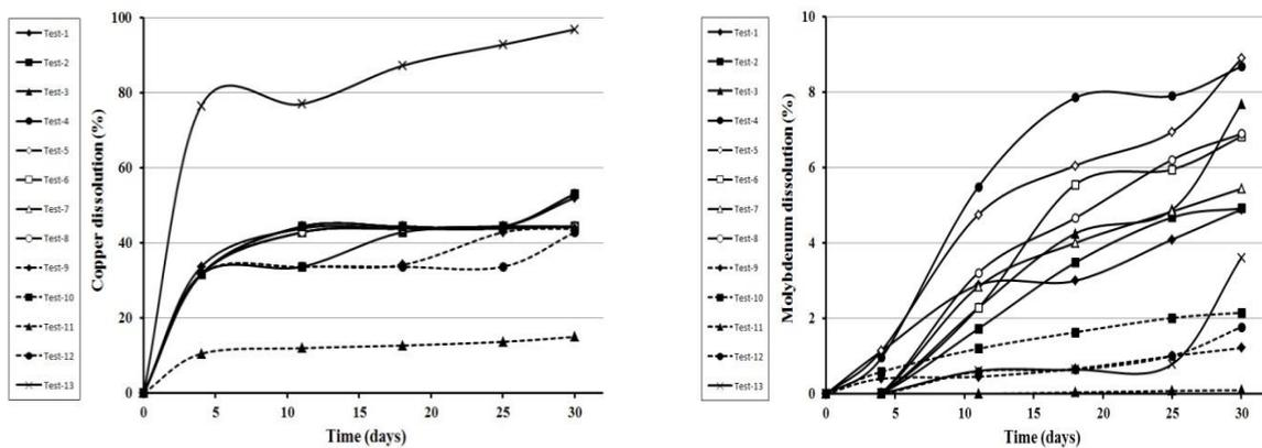
Figure 12. The Cu and Mo extraction in mesophilic bioleaching test
