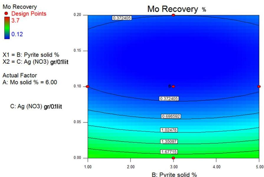
Figure 10. Influence of pyrite percent (%), and silver ion concentration ( $\text{gr l}^{-1}$ ) on the molybdenum dissolution.
