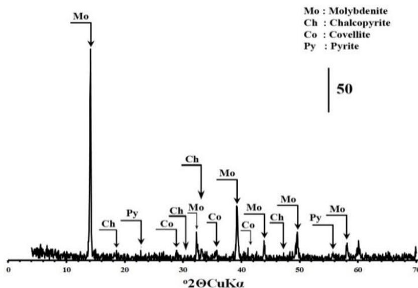
Figure 1b. X-ray diffractogram of molybdenite concentrate with chalcopyrite, covellite and pyrite minerals as impurities.
