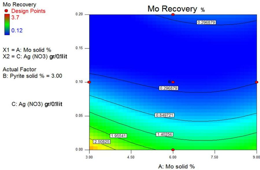
Figure 9. Influence of molybdenite concentration (%), and silver ion concentration ( $\text{gr}^{-1}$ ) on the molybdenum dissolution.
