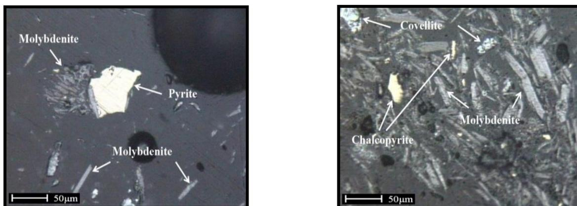
Figure 1a. Mineralogical observations from Molybdenite concentrate with chalcopyrite and pyrite minerals
