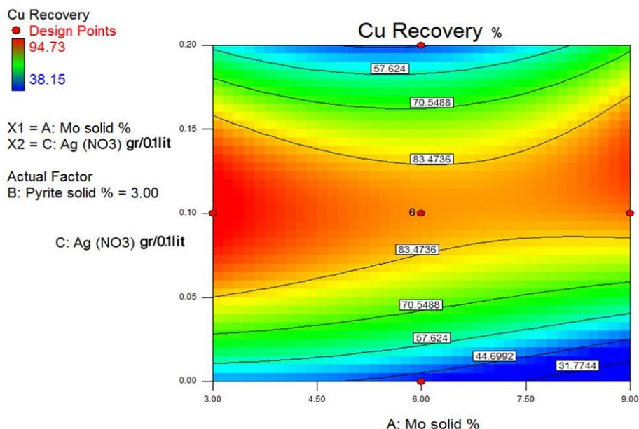
Figure 7. Influence of molybdenite concentration (%), and silver ion concentration ( $\text{gr l}^{-1}$ ) on the copper dissolution.
