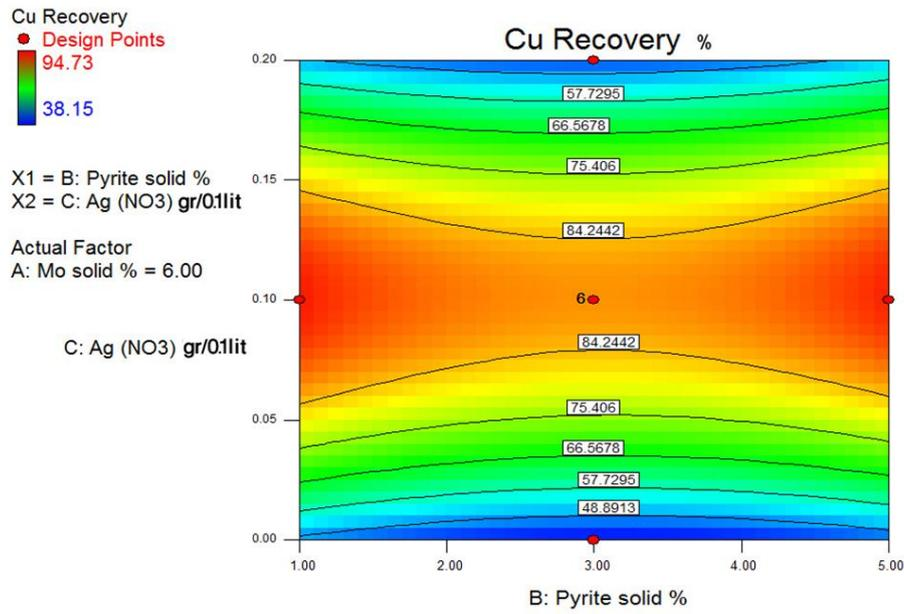
Figure 8. Influence of pyrite percent (%), and silver ion concentration ( $\text{gr}^{-1}$ ) on the copper dissolution.
