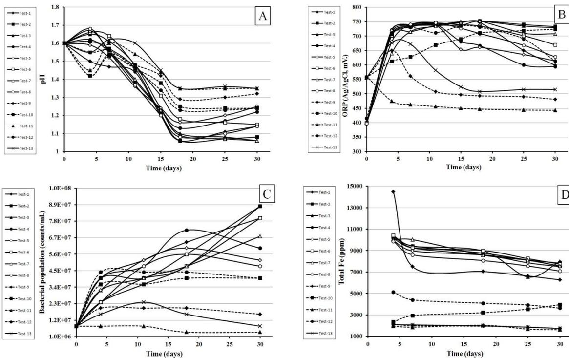
Figure 11. The changes of pH, Eh, cell counts and Total Fe in the mesophilic bioleaching tests
