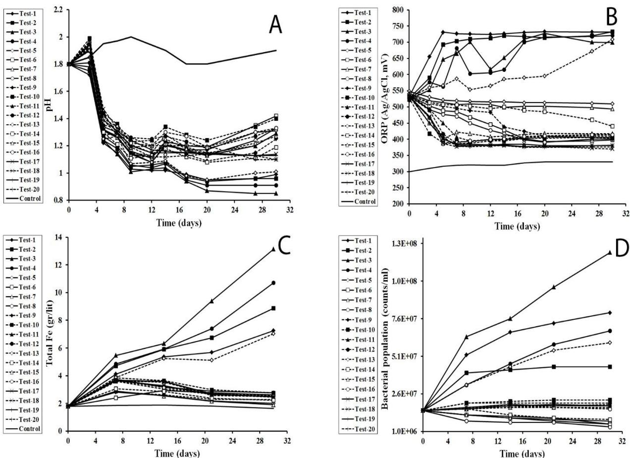
Figure 4. The changes of pH, Eh, Total Fe and cell counts in the mesophilic bioleaching tests
