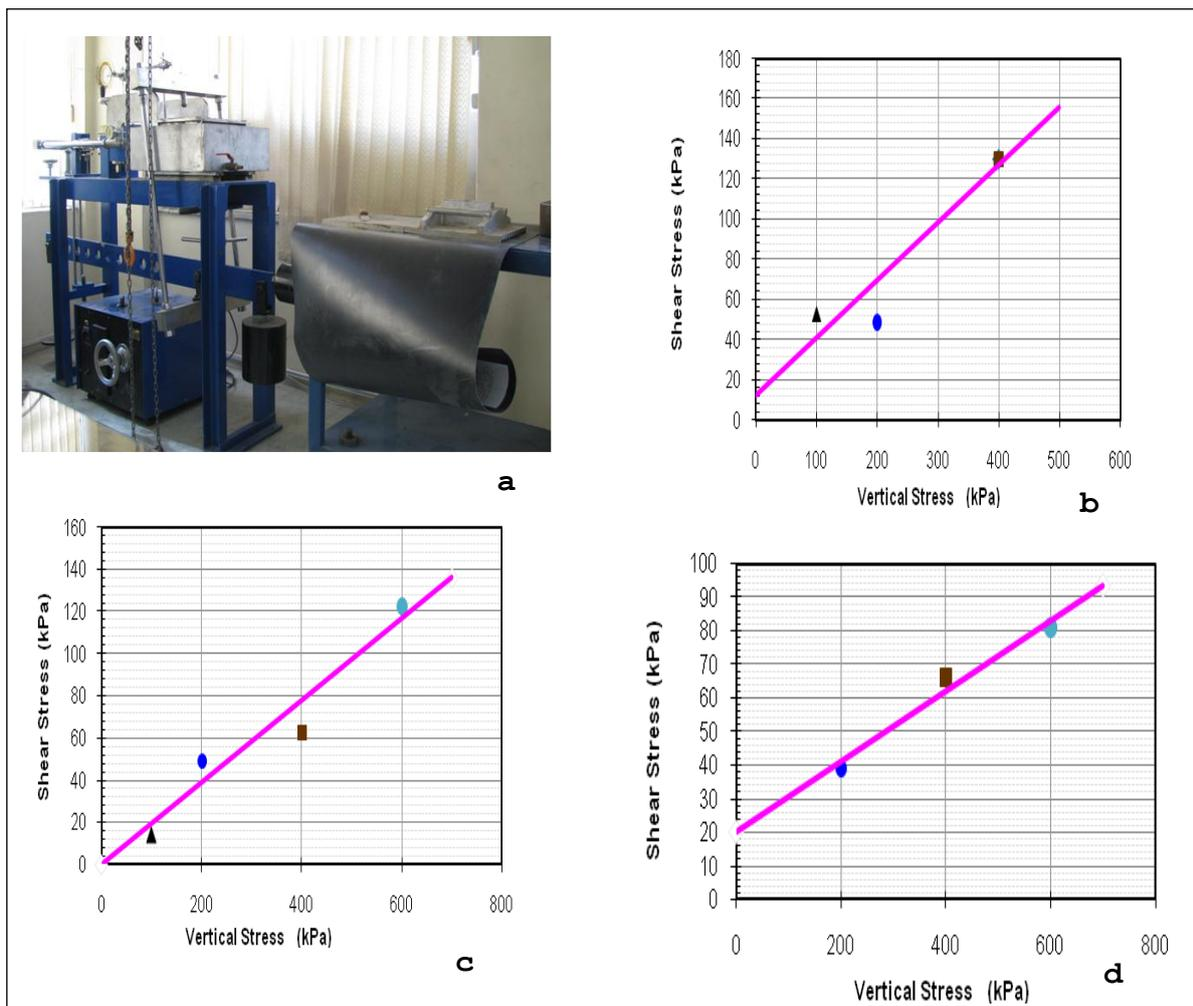
**Figure 4. Direct shear tests results of the heap beds materials a) Direct shear test machine for determining shear strength parameters between geosynthetic-soil and geosynthetic-geosynthetic materials, b) Between compacted fine composite soil and GCL, c) Between GCL– GM, d) Internal slide in GCL**
