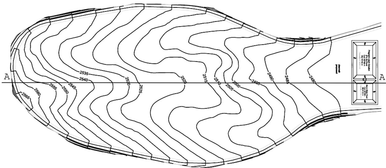
Figure 7. Miduk heap foundation topography after earthwork
