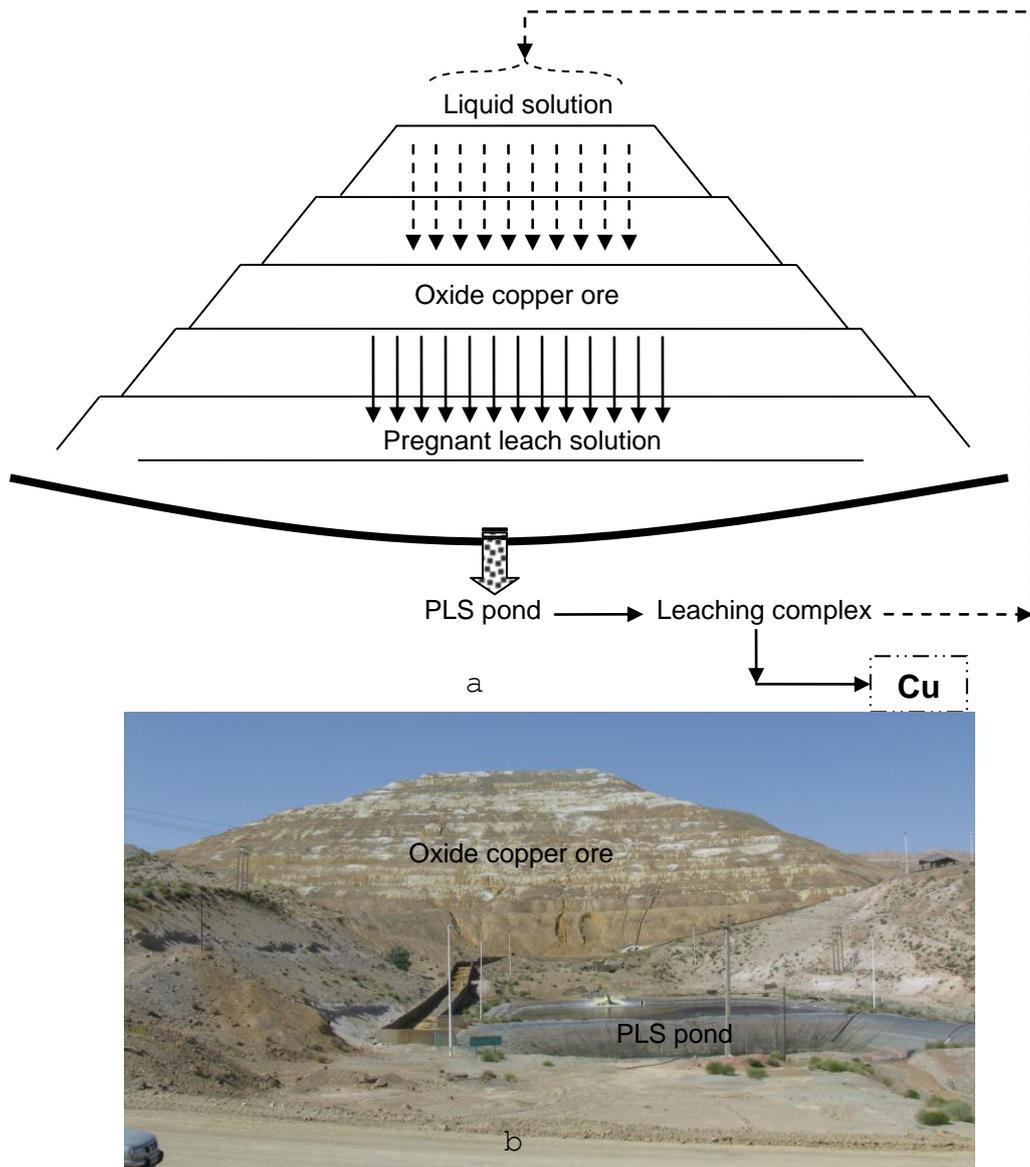
Figure 1. Heap leaching structure: a) schematic view; b) "Sarcheshmeh" copper heap leaching structure 1
