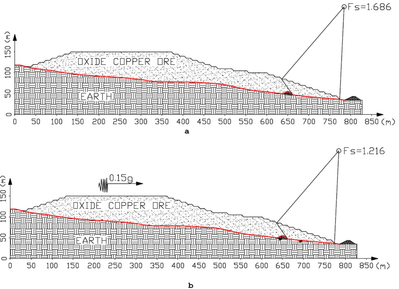
**Figure 10. Stability analysis for Miduk heap after stabilization at section A-A**
