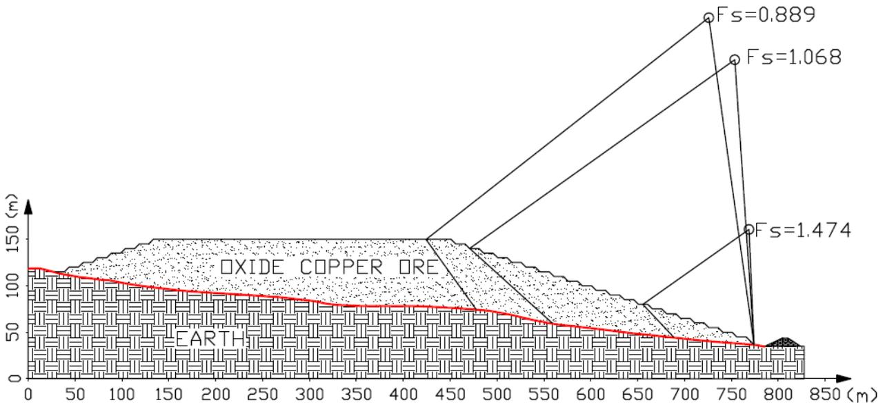
**Figure 8. Stability analysis of Miduk heap after earthwork in A-A section**
