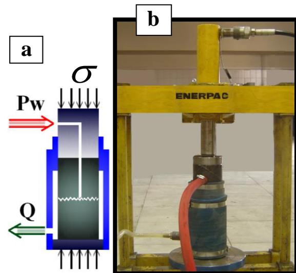
Figure 1: a) Schematic of the jointed rock sample surrounded by a cover subjected to the axial load
