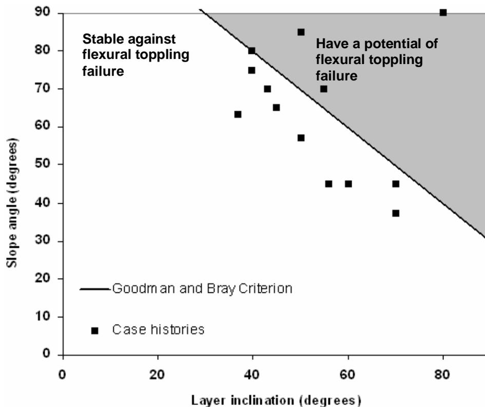
Figure 3: Assessment of the case histories of flexural toppling failure on the basis of Goodman and Bray method
