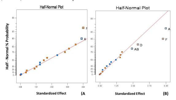
Figure 2: Standard effects on log-normal curve related to response of ash percentage of concentrate. A: ground sample, B: non-ground sample
