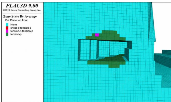
Figure 16. Condition of Room Roof Zone After Initial Step - Section 3-3.
