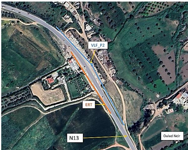
Figure 8. Aerial view of the My Idress site showing VLF-ERT geophysical profile locations.
