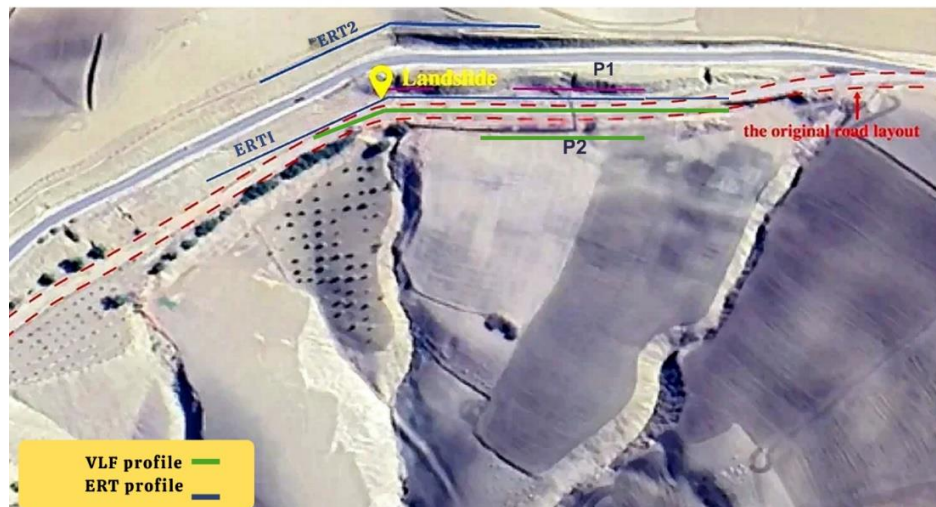
Figure 4. Aerial view of the My Yaacoub site showing the original road layout and VLF-ERT geophysical profile locations.
