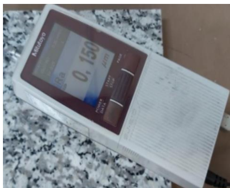
Figure 4. Roughness tester device used in this study.
