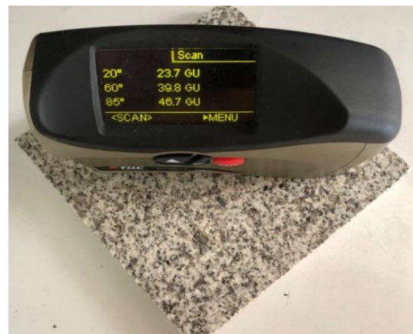
Figure 2. The gloss meter used in this study.
