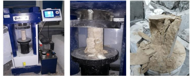
Figure 6. Example of a compression test performed on a phosphate specimen.
