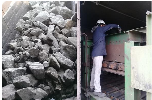
Figure 2. AG mill feed sampling at the apron feeder.
