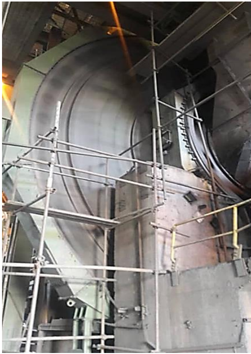
Figure 1. Autogenous mill in Line 3 of the Gole-gohar complex.
