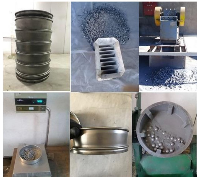
Figure 3. SPI testing procedure and equipment.
