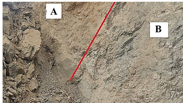
Figure 1. An illustration of the locations of ore types A and B in Khanjar's mixed sulphide-oxide ore.
