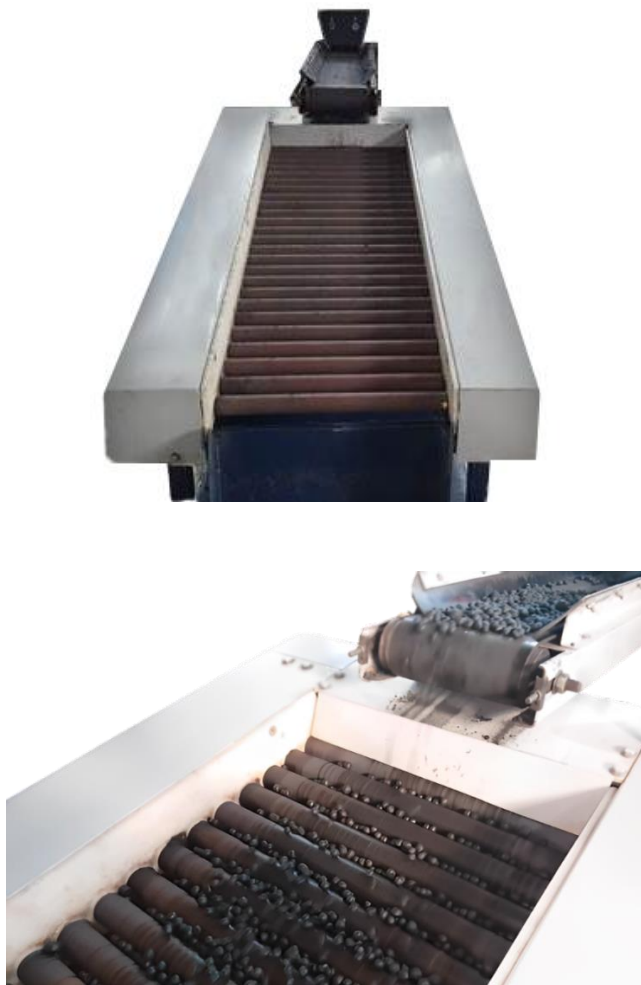
Figure 4. The laboratory roller screen for experimental tests of the green pellet classification.
