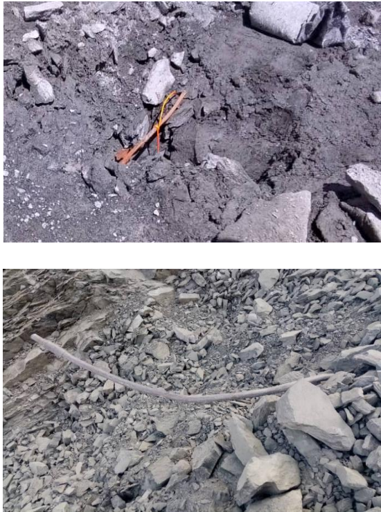
Figure 4: Field photographs showing (up) a collapsed blast hole due to poor ground conditions and (down) a lost drill steel rod embedded within fragmented muck at the Eureka Delta Gold Mine.
