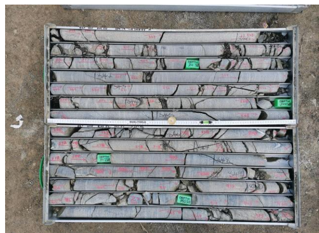
Figure 3: Drill core tray from the Eureka Delta Gold Mine showing intersecting joints, variation in fracture persistence, and visible alteration zones.
