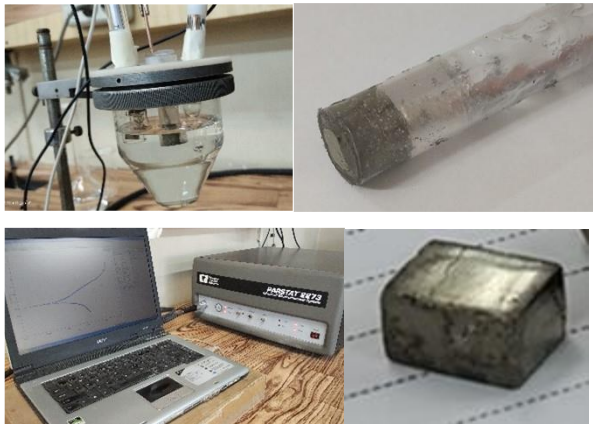
Fig. 2. The preparation steps of pyrite (WE) working electrode.
