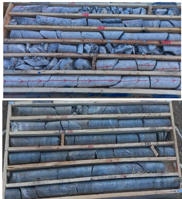
Fig. 2. Several exploratory cores from drilling operation in the Sungun mine.
