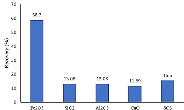
Figure 5. The recovery of iron and other important elements in the concentrate of the magnetic separation experiment at a field intensity of 6000 Gauss.
