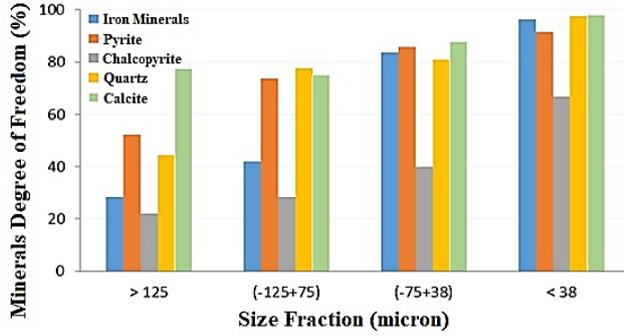
Figure 3. Changes in the degree of freedom of the main mineral of the tailings dam in different size fractions.
