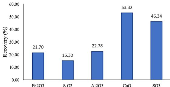
**Figure 6.** The recovery of iron and other components in the concentrate obtained from the flotation on the tailings of the magnetic separation experiment.
