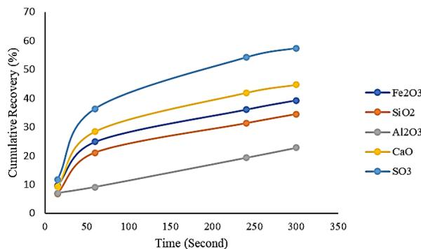
Figure 4. The results of the gravity concentration experiments using the spiral equipment.
